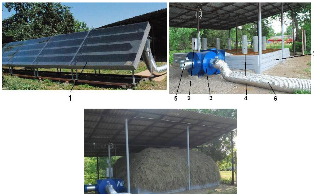
Fig. 2. Experimental model of the installation for fodder ventilation, IVF: 1 – assembled solar panel; 2 – electrical installation; 3 – ventilation equipment; 4 – ventilation tubes; 5 – intake flanges with electric motor; 6 – piping for hot air circuit; 7 – drying/storage platform
